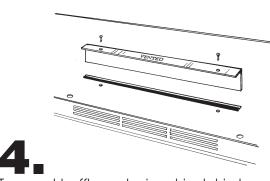
Turn vent baffle and reinsert in slot in top of range hood so that the word "Vented" is facing up. Fasten vent baffle with screws.
